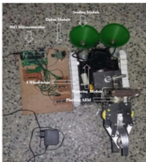
Figure 4. Labelled diagram of the smart arm
